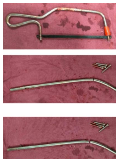
Figure 10: Mini Hacksaw blade mounted on Handle and Removed Bent Nail (cut into two Pieces)
